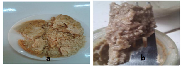
Figure 4. Alkali extracted ash from banana stalks (a) and wood ashes (b).
